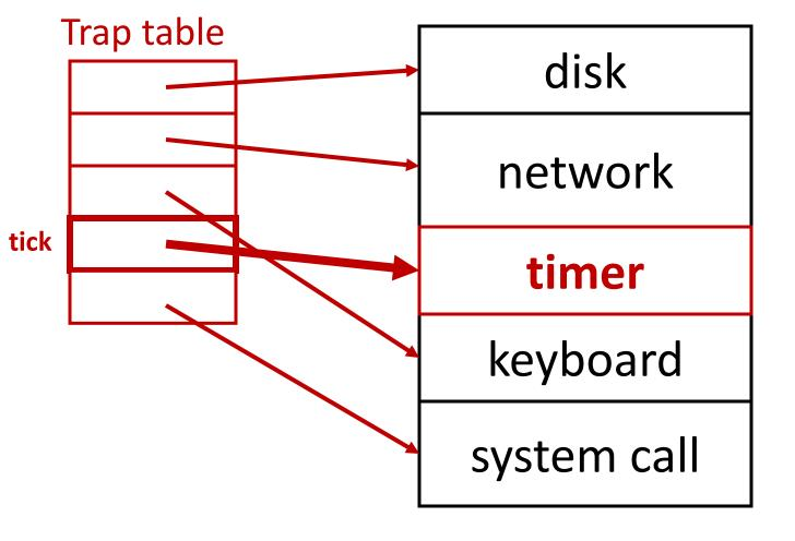
Use array of function pointers to locate OS functions (Hardware knows this through **lidt** instruction)
