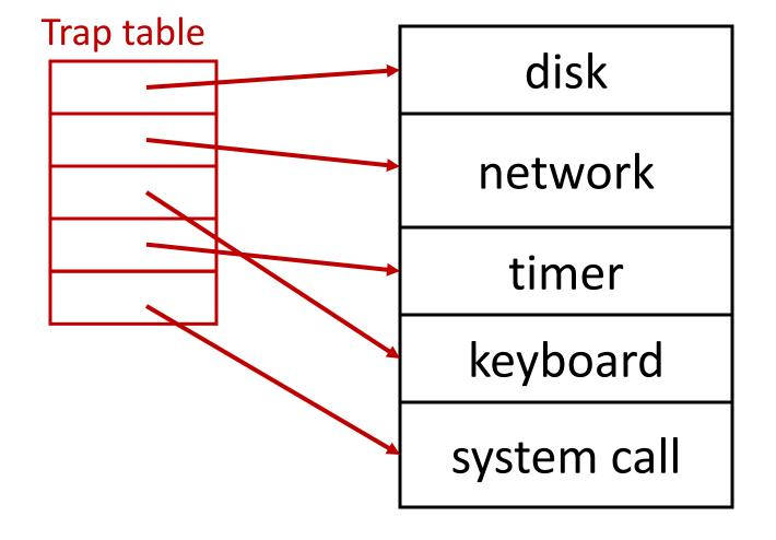
Use array of function pointers to locate OS functions (Hardware knows where this is)
