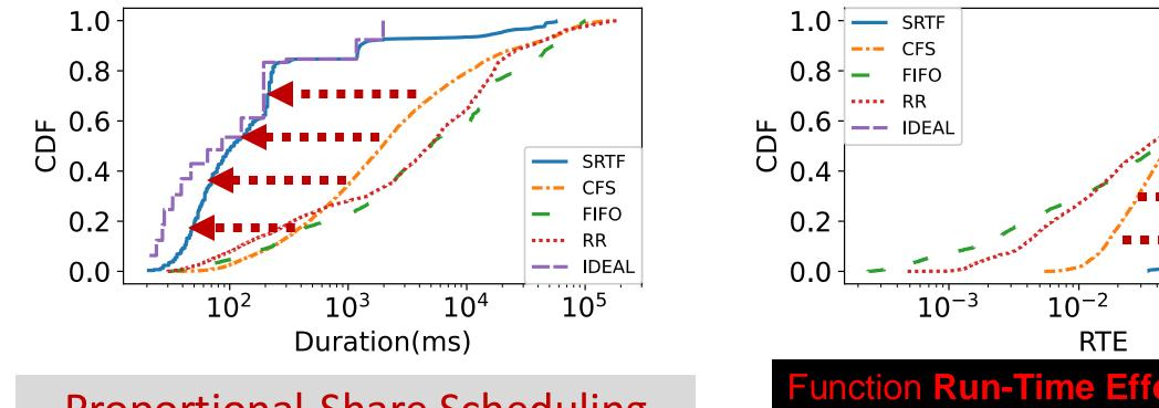
Proportional-Share Scheduling offer poor performance Function Run-Time Effectiveness = Service time / Turnaround time CFS frequently preempts functions, causing longer waiting time (w/ smaller RTEs)
