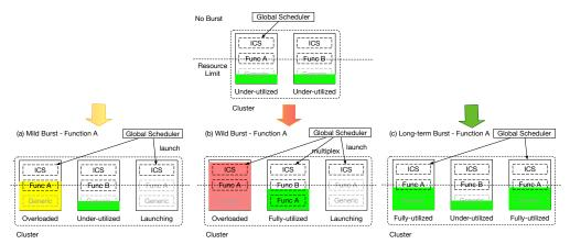
**Figure 2:** Overview of multi-phase auto-scaling scheme: (a): Transient scaling-up offers a temporary solution to mitigate the impact of mild burst, while waiting for the new containers to be launched from background; (b): Container multiplexing effectively serves wilder burst; (c): When the scaling-out process is finished, distribute the persisting burst to the new containers.
